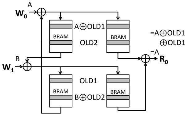
**Figure 3:** A 2W/1R memory implemented using XOR, with example data values. Note that only data wires are shown, not address wires.  $W_0$  stores the value  $A$  XOR'ed with the old contents of the other bank ( $OLD1$ ). Similarly,  $W_1$  stores the value  $B$  XOR'ed with the old contents of the other bank ( $OLD2$ ). Reading the location containing  $A$  computes  $(A \oplus OLD1) \oplus OLD1$  which returns  $A$ .
