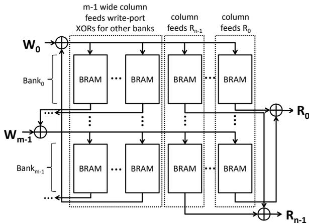
**Figure 6: A generalized  $mW/nR$  memory implemented using XOR. Each write port requires a bank (row) of BRAMs. A column of BRAMs is required for each read port, as well as a column for each of one less than the total number of write ports.**
