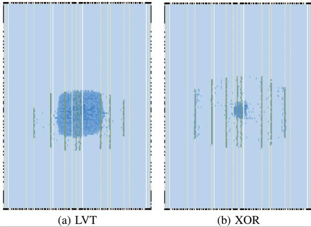
**Figure 8: Circuit layout of 8192-deep 2W/4R memories for (a) LVT and (b) XOR designs, as rendered by Quartus. The thin columns are BRAMs or DSPs (darkened indicates in-use), the dots and dot-clouds are ALMs.**
